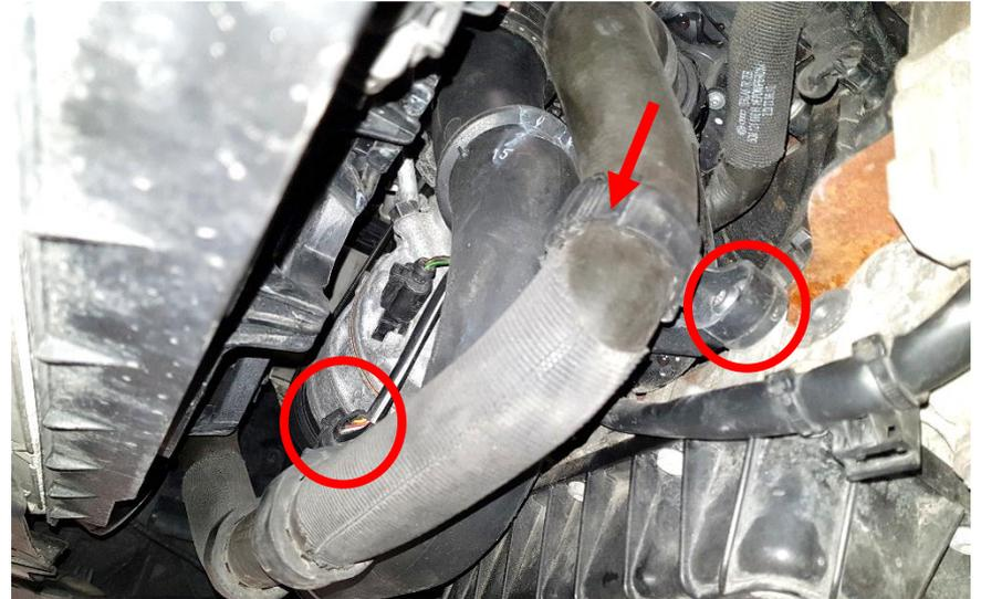
11. Install the OEM screws and rubber bushings (4pcs) from the OEM pipes on the do88 pipes. Also remove the sensor from the OEM pipe and install it in the do88 pipe with the included screws.
