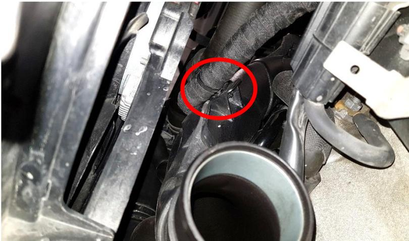
8. Remove the air intake scoop by removing 2x Torx T25 and unclick the radiator hose.
