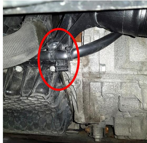
7. Disconnect the cable from its bracket on the intercooler inlet pipe. Then remove the pressure pipe from the car, remove it downwards.
