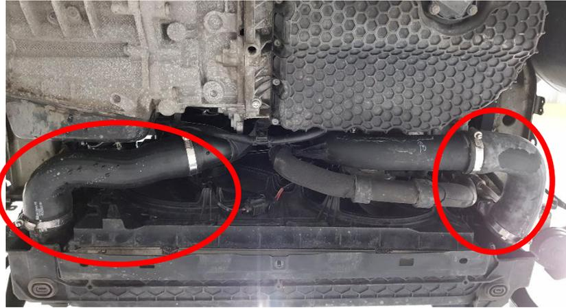
6. Disconnect the cable from its bracket on the intercooler inlet pipe also loosen 1x Torx T30.
