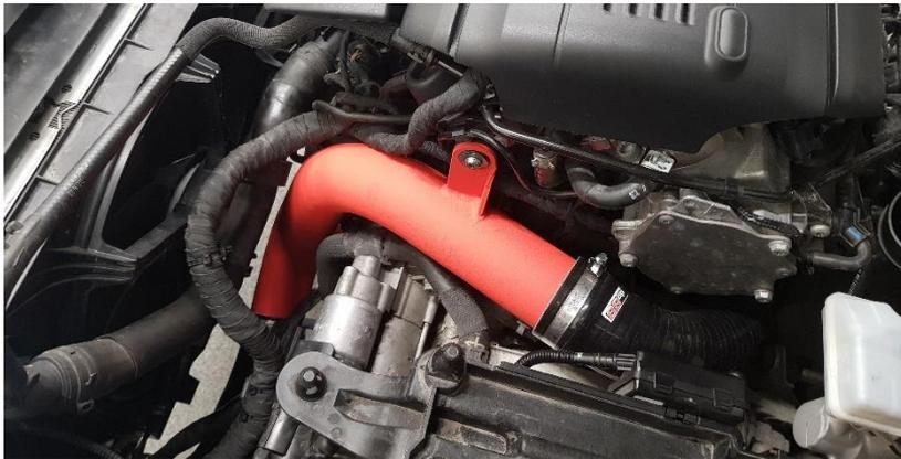
13. Put the throttle body hose on the intercooler pipe, but don't tighten the clamp yet. Then install the pipe in the car. Just loosely tighten the two screws now.
