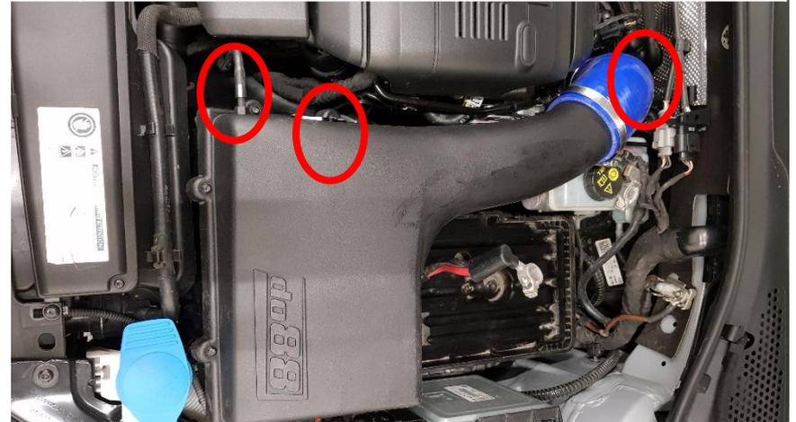
3. Loosen 1x Torx T30 screw at the pressure pipe bracket and 1x hose clamp on the turbo outlet. Also disconnect the small plastic box from its bracket on the battery tray.
