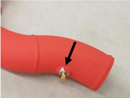
14. Put the turbo outlet hose on the other intercooler pipe, but don't tighten the clamp yet. Then install the pipe in the car. Just loosely tighten the two screws now.
