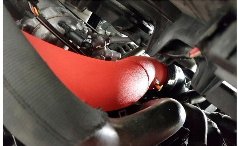
15. Install the intercooler in- & outlet hoses. Adjust position on all hoses then tighten all clamps and screws. Reinstall all other parts in reverse order.
