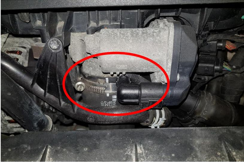
10. Disconnect the sensor cable connector, 2x Torx T30 screws. Also unclip the lower radiator hose from its bracket on the pressure pipe. Then remove the pipe.
