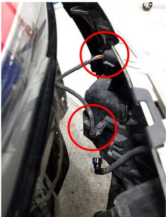
10. Unclip the hood cable joiner located over the left head light. Important! Remember to reconnect during re-installation, otherwise you can't open the hood.
