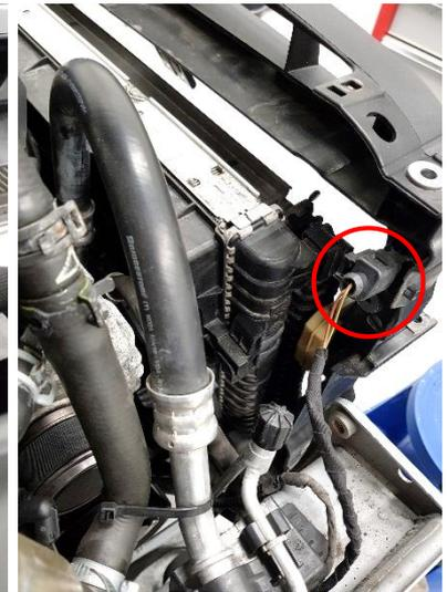
15. Disconnect the cable connector for radar, temperature sensor and both horns. Make sure to loosen all wires from the radiator support so it can be removed from the car.
