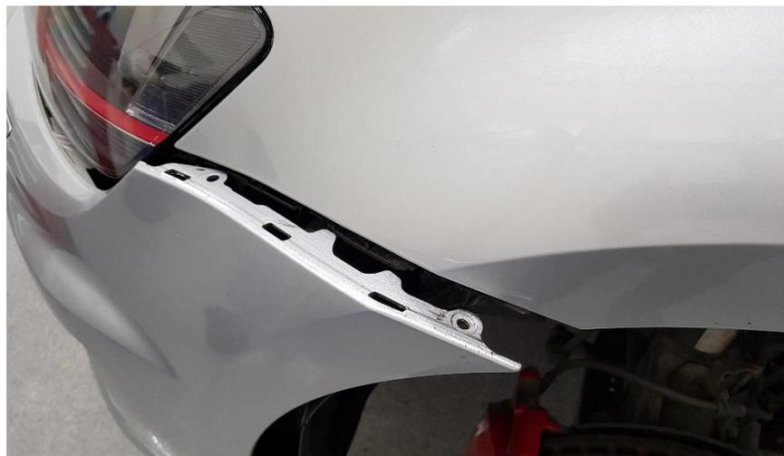
9. Gently lift the bumper forward a little bit, then disconnect all cable connectors.
