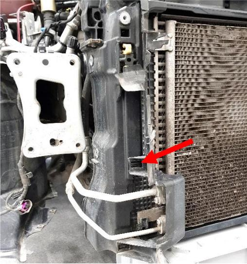
**20.** The intercooler and radiator assembly is fastened with the two large plastic clips. Release these with a flat blade screwdriver. Gently press the intercooler backwards while pressing on these clips.
