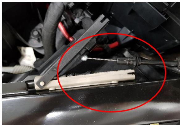
11. Remove 3x Torx T30 for the brackets above both head lights. Remove both brackets, on the left side you need to disconnect washer fluid pipe and cable hood lock joiner.
