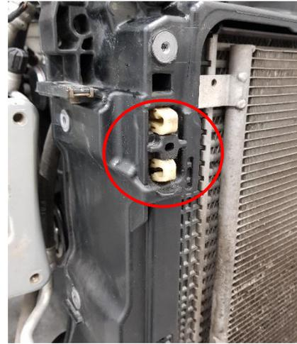
**21.** When you have released the two clips in step 20. Disconnect the AC-condenser from the intercooler. Do this by pressing the two top plastic tabs while lifting it upwards. Strap the AC-condenser to a support until re-installation.
