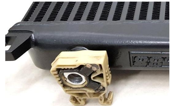
25. Cut the top right bracket on the AC-condenser. Cut on the outside of the raised rib.
