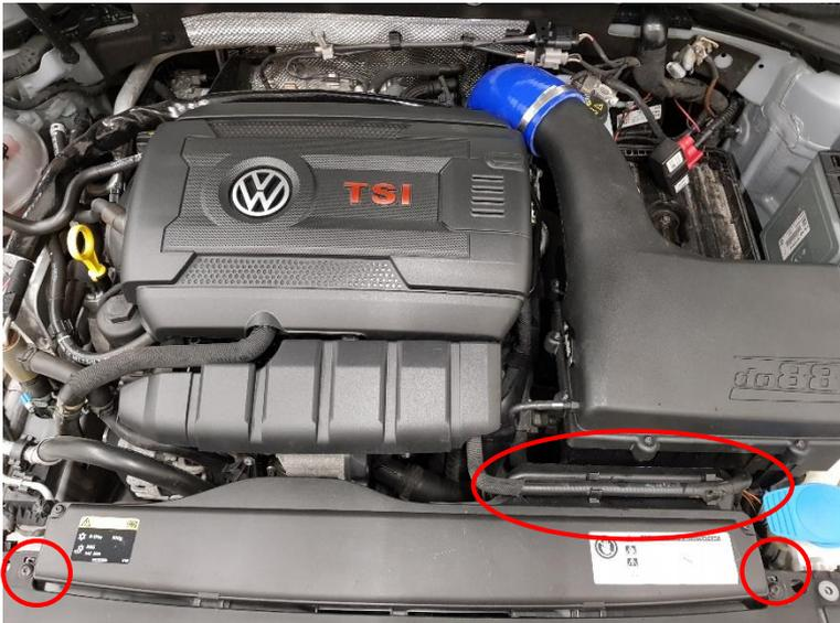
14. Disconnect the marked cable connectors on the photo below. They are located on the backside of the radiator support. Loosen the cables from the radiator support.
