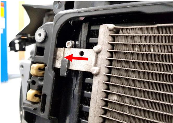
26. The left sides air guide needs to be slightly trimmed. Cut the plastic with a plier on the marked locations.
