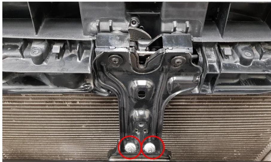
**18.** Now place a steady support underneath the radiator pack. On both sides remove 4x Hex 16mm screws and 2x Torx T30 screws. Then with the help of a friend remove the crash bar from the car.
