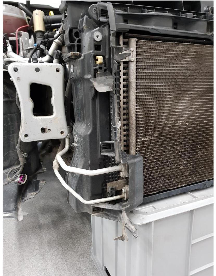
**19.** Remove the plastic air guides on both sides. Press the plastic clips downwards with a flat screwdriver.
