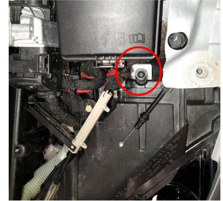
13. Remove the air intake scoop by removing 2x Torx T25 and disconnect the radiator hose from clips.
