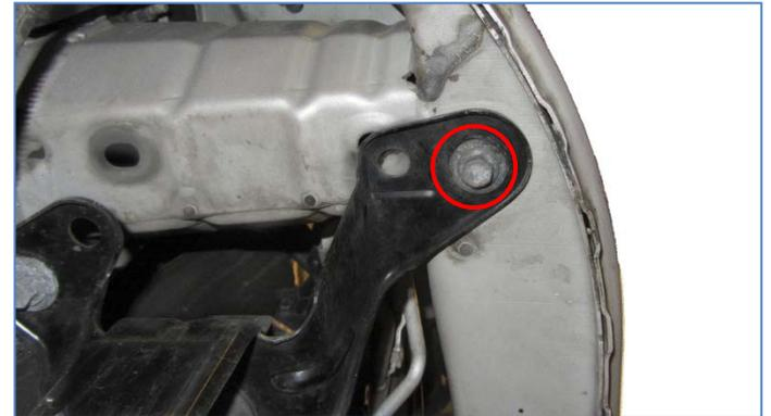
**14.** Install left and right intercooler bracket with 1pc M8x30 flange head screw and a thick washer each. The thick washer installs between the bracket and the radiator bracket. Do not tighten screws now as brackets should be adjustable.
