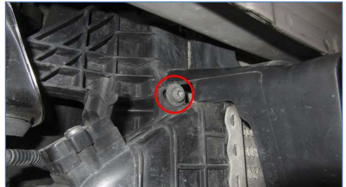
**12.** Remove the sensor from the OEM intercooler by removing its Torx T25 screw and pull it up from the intercooler.
