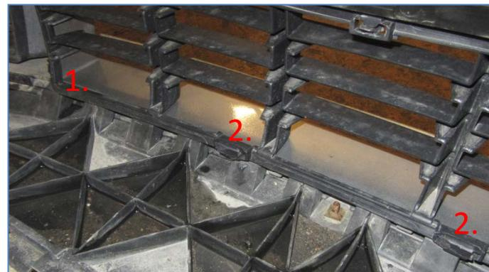
**19.** One of the brackets on the left hand plastic fog light frame needs to be trimmed at the red line to avoid interference with the intercooler tank.
