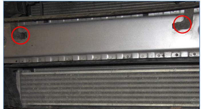
8. Remove the upper air ducting by pulling it forward to remove it from fasteners and air inlet guide in the upper part of the guide. Then tilt the upper part out of the car and remove.
